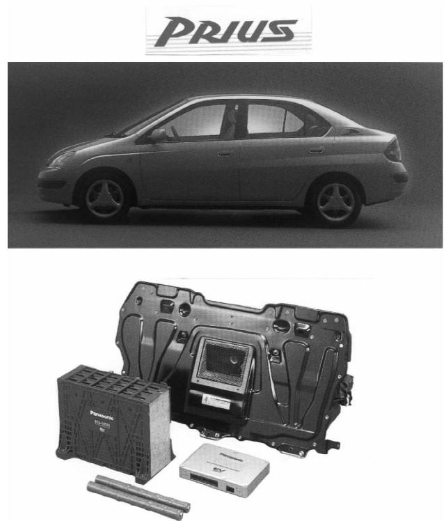
Fig. 3. Hybrid electric vehicle Toyota “Prius” and its battery pack.
